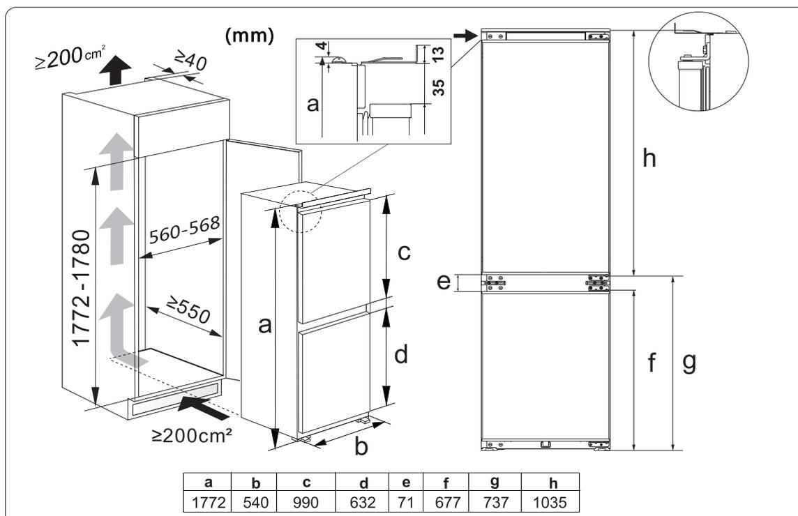
Please ensure there is enough space of the cabinet for the refrigerator, it is necessary for the installation, repairs and air circulation. Before installation, please confirm that the cabinet size.
